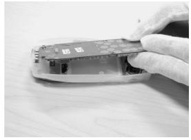
The PWB (shown at left) can be removed by lifting it up from the guide pins in the D-cover.
