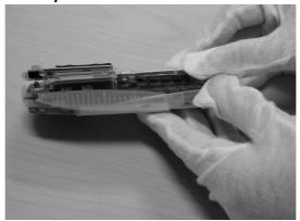
Note: Make sure that the LCD assembly is completely loose from the D-cover snaps to minimize the risk of bending the LCD board.
