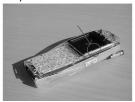
Insert a nonconductive tool on the side of the LCD and carefully snap the LCD assembly out from the D-cover.
