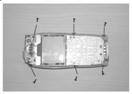
Remove the six screws using a nonconductive screwdriver (Presicion Torx Driver T6 Required).
